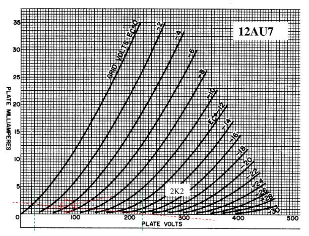
**4.3 12AU7** *tone recovery section.* 12AU7, V2B; VS4 = 232V; Va=100V; Rk=4k7; Vk=4.8V; Ia=1.0mA; RLdc=120k.
